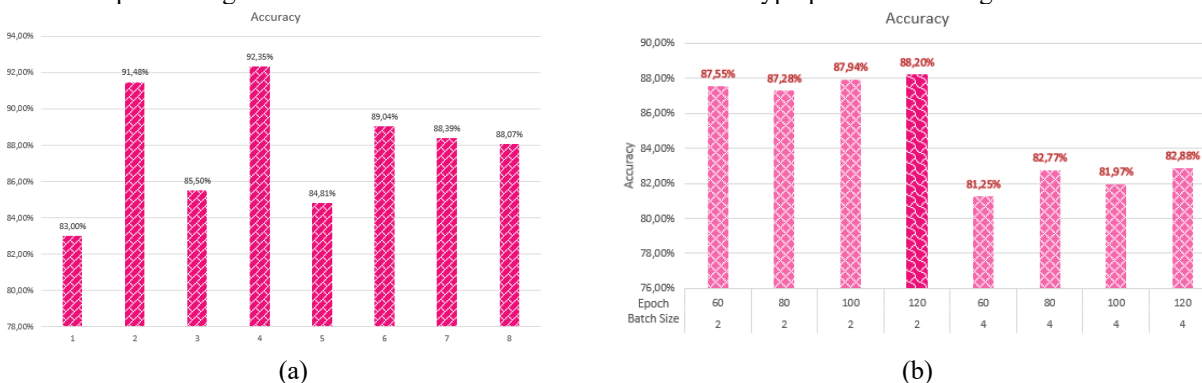
Fig. 3. the RetinaFace training results using (a) the ResNet-152 (Resnet), (b) MobileNet V1 (0.25) (Mnet)
