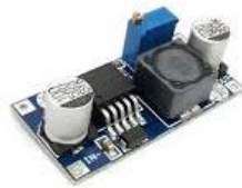
Source : techdelivers.com Figure 3. Step Down Regulator DC
