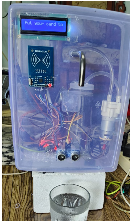
Gambar 7. Prototipe smart water dispenser berbasis Internet of Things
